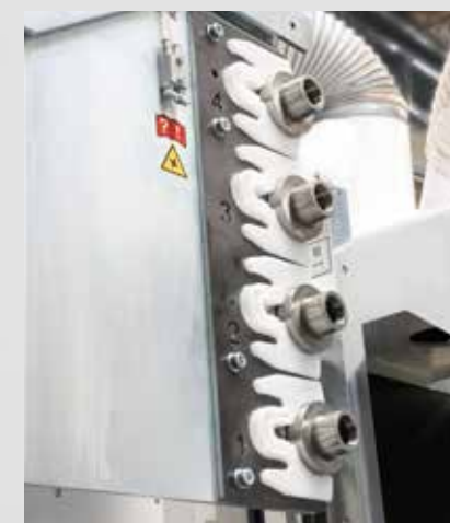
4-fold tool changer ▪ 4 tool positions are provided in the tool changer system for customized machining. ▪ Simple changing by coupling the changer to the inside of the machining area. ▪ All the tools that are important to you can be stored and managed in our tool management system toolManager. They can be easily transferred to the machining process using drag & drop.
