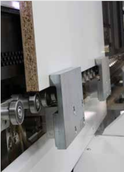
CNC-controlled collet system with 2 collets Vacuum-free fixing and precise positioning of workpieces. You save 100 % vacuum force here.
