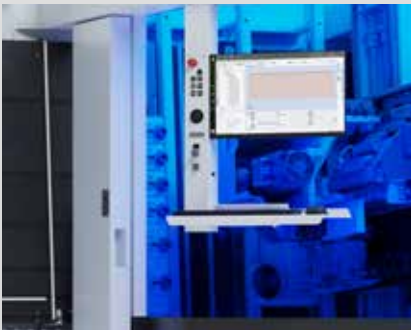
Step 4: ▪ Comparison of the determined values with the program data: ▪ Tolerance of values < 5 mm - program is continued. ▪ Tolerance of values > 5 mm - program is stopped, hint to the operator to make the corrections.
