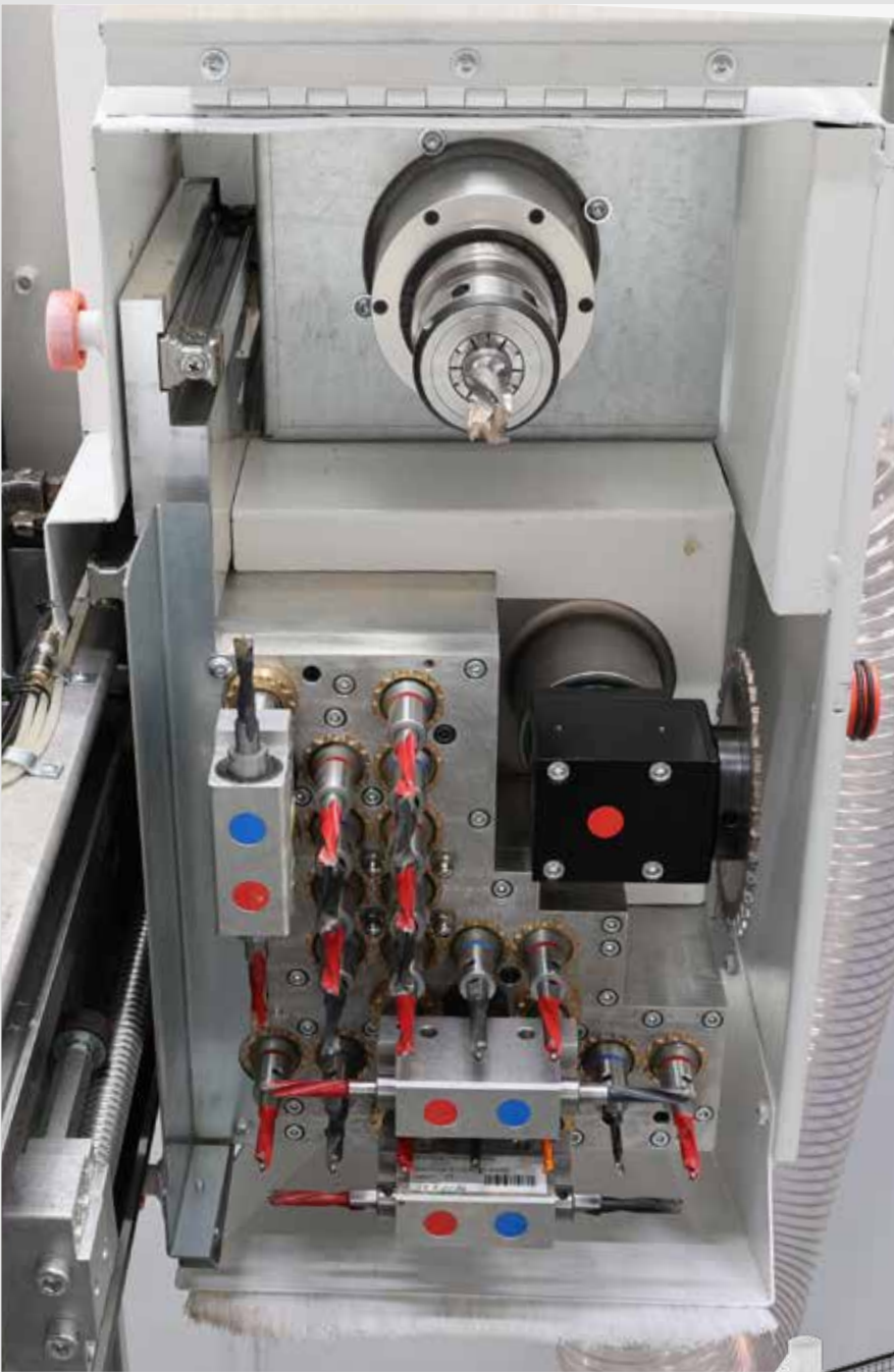
Space-optimized machining The tool interface is arranged above the drilling gear to save space. The reduced installation space is fully utilized for flexible machining.
