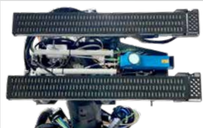
A camera system assists with the identification and decoding of the stack pattern
