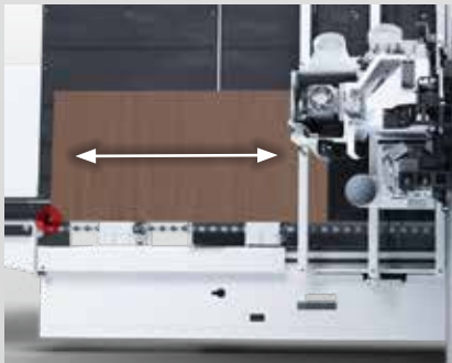
Step 2: ▪ Control of the workpiece by sensor technology in X-direction. Depending on the workpiece size, the shortest path to the next sensor is selected.
