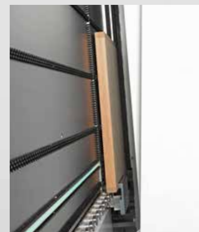
Easier material handling By utilising gravity with 5° inclination.
