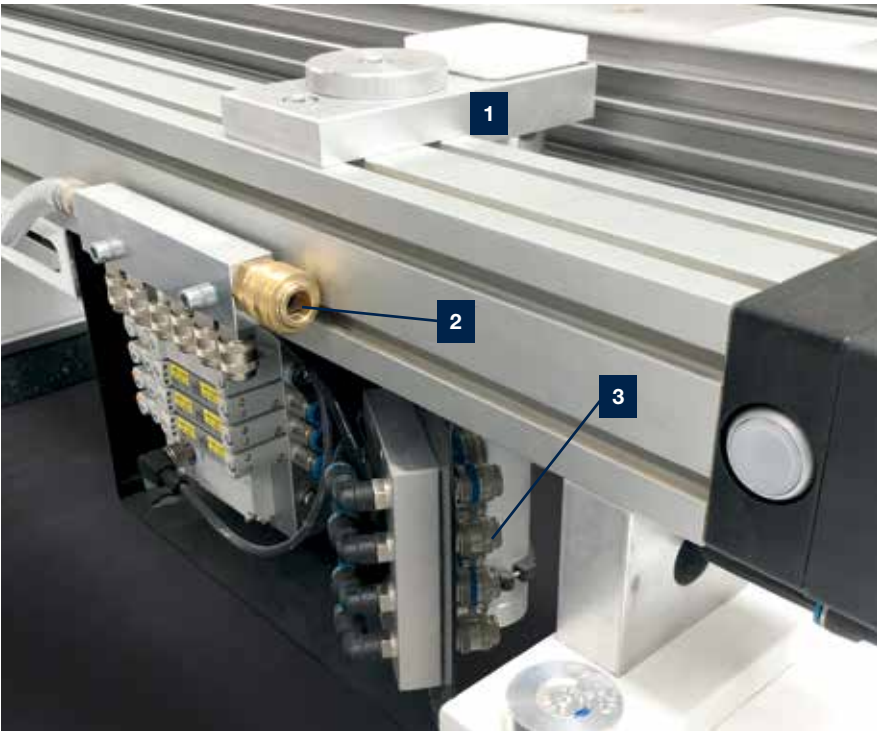
Base plate module for mounting on the consoles as the basis for special clamping fixtures.
