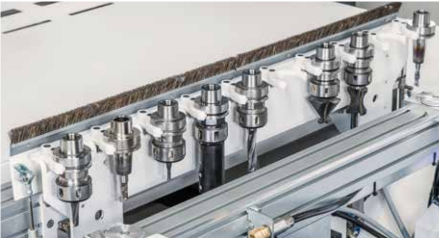
Linear changer ▪ Additional tool change magazine with 10 places (optional), on the left side of the machine frame
