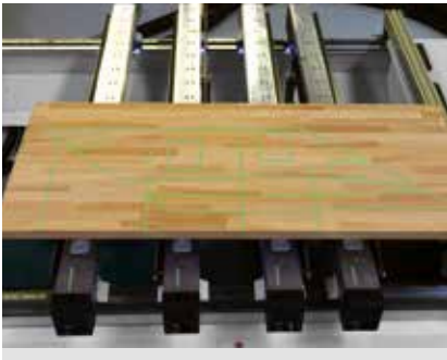
Laser projection of the clamping equipment and the workpiece contour for optimal utilization and simple positioning of unprocessed parts that cannot be aligned on the stops.
