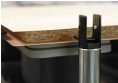
Stops for coating ply overhang (optional) Ensures easy positioning in the case of coating ply overhang (e.g. veneer)
