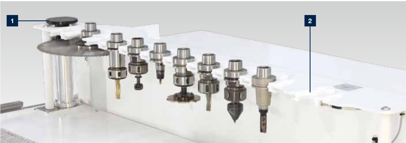
Linear changer ▪ Additional tool change magazine, with 10 slots and integrated tool transfer station, laterally mounted. ▪ One slot is prepared to accommodate a saw with a diameter of 350 mm.
