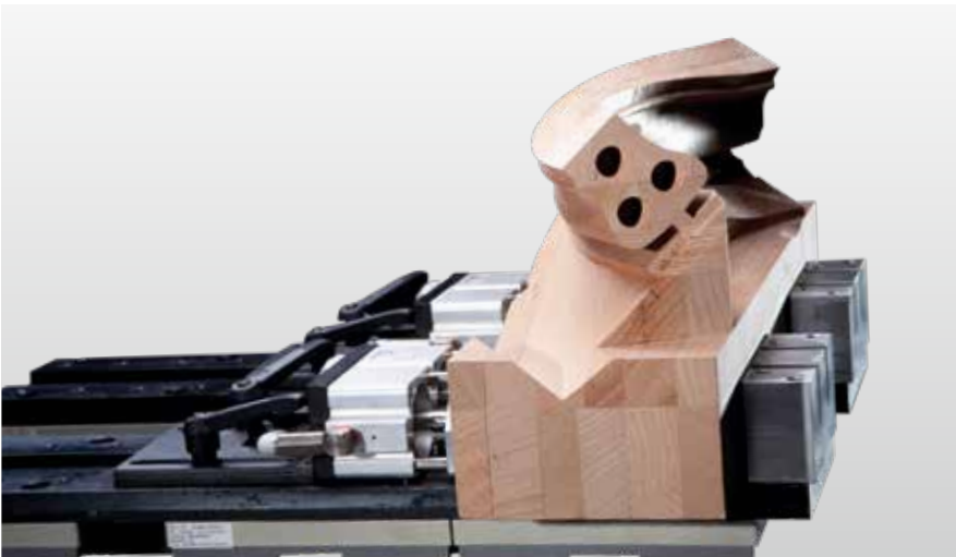
Clamping device Uprights and staves can be securely clamped in no time using this clamping device
