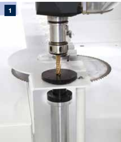
Tool length control (optional) ▪ Suitable for length measurement of shank tools ▪ Following the tool change via the tool pick-up station a tool length control is carried out and compared with the integrated tool database
