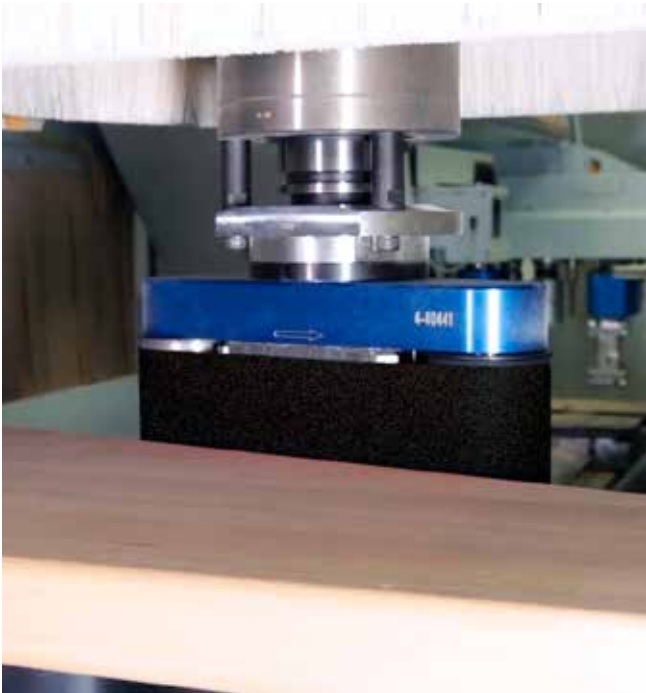
Pneumatic interface – the interface with 3-way support on all C-axes and optionally on the DRIVE5CS enables the use of traced units, e.g. for precise rounding off at the top and bottom no matter the thickness tolerances.
