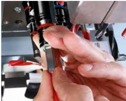
Quick-change system for a drill change without tools to reduce setup times.
