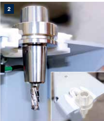
Tool pick-up station ▪ Safe and quick fitting of the tool change magazine ▪ High safety by sensor monitoring if the tool pick-up station is free or occupied
