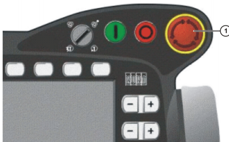
Fig. 5-3: EMERGENCY STOP button on the KCP
