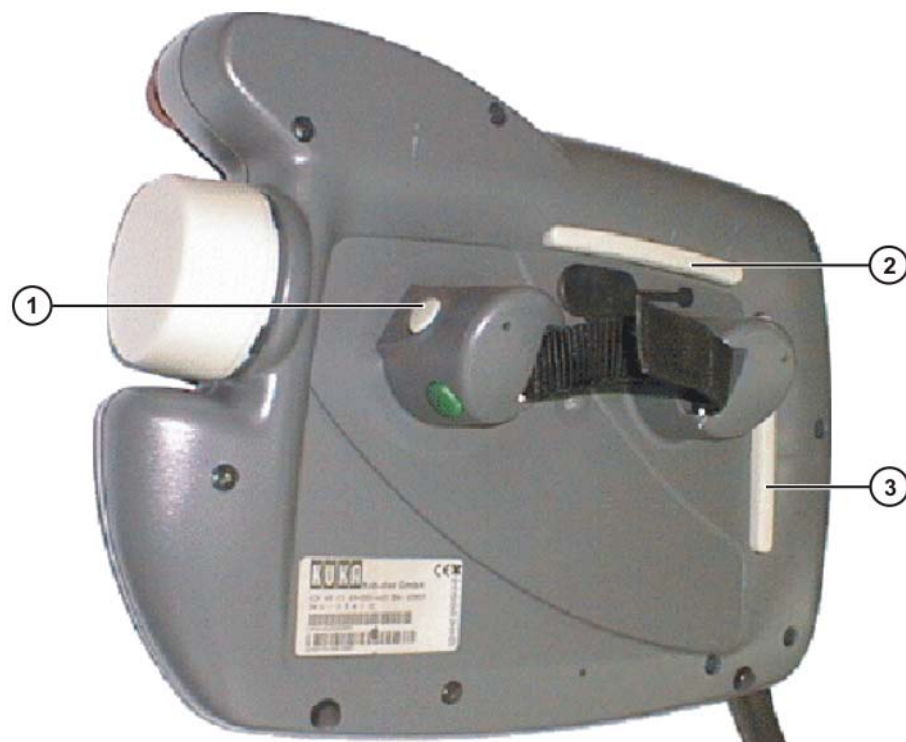
Fig. 5-4: Enabling switches on the KCP
